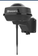
Transmits RTK-GNSS signals between the Automower® 550 EPOS mower and guidance satellites. The mains powered reference station is required for EPOS to function and can serve multiple EPOS units per installation. Work area up to 500 metre radius.
