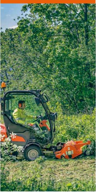
A full range of attachments designed to increase the flexibility of your investment whilst allowing true all year round use. The range consists of PTO and hydraulic controlled front mount attachments all designed for full time commercial use and optimised for use with the P 500 Series.
