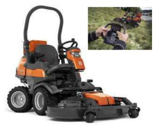
Front-mounted petrol ride-on lawn mower, built for commercial use. Compact and versatile with articulated steering, All-Wheel Drive and a Kawasaki engine with Electronic Fuel Injection for enhanced power and torque. Intended for facility management companies, sports clubs and for contractors who want a manoeuverable ride-on solution for year-round duties in complex areas. Adapted for high capacity cutting decks up to 137cm.
