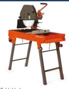
The TS 400 F is an efficient universal masonry saw with high cutting capacity for all kinds of bricks and building blocks. You can easily plunge or bevel cut at 45 degrees for maximum versatility. The robust single-piece frame with integrated conveyor rails gives great rigidity and provides longer product life.
