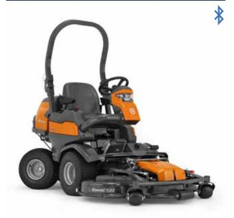
Front-mounted petrol ride-on lawn mower, built for commercial use. Compact and versatile with articulated steering, All-Wheel Drive and a powerful engine from Kawasaki. An electric attachment lift enables efficient and comfortable work. Intended for facility management companies, sports clubs and for contractors who want a maneuverable ride-on solution for year-round duties in complex areas. Can be equipped with 112cm and 122cm combi cutting decks.
